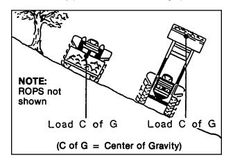
When working on side hills, **DO NOT RAISE LOADER TOO HIGH.** Keep an eye on terrain changes. Keep load low.
