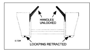
Figure 2. Quick Attach Coupler Handles - Unlocked
