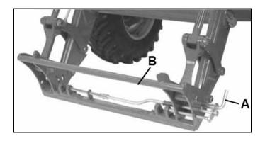
NOTE: Most latches automatically close on global carrier.
