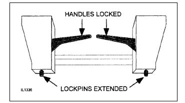
Figure 3. Attachment Coupler Handles - Locked
