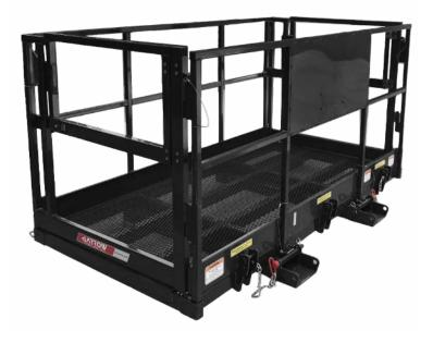
Arrow's new work platforms exceed OSHA/ANSI Standards B56.6-2021 and CSA B335, ensuring top-tier safety. With easy, tool-free assembly, each platform features standard safety restraint tie-downs rated for 3,600 lbs, heavy-duty hinges and latches, and self-latching/self-closing doors. Rated for a 1,000 lb capacity, these platforms offer secure and reliable support for both men and materials.
