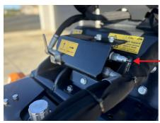
Sequence valve (To engauge saw)\*Preset factory setting DO NOT ADJUST\*
