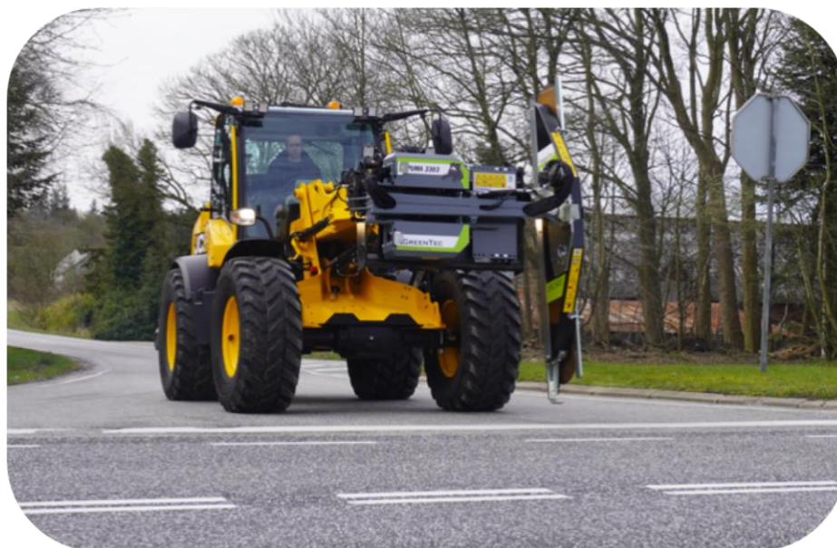
Example of transport position: Lights free on the vehicle, clear view, with safety devices mounted on the attachment tool, facing the vehicle for maximum traffic safety.
