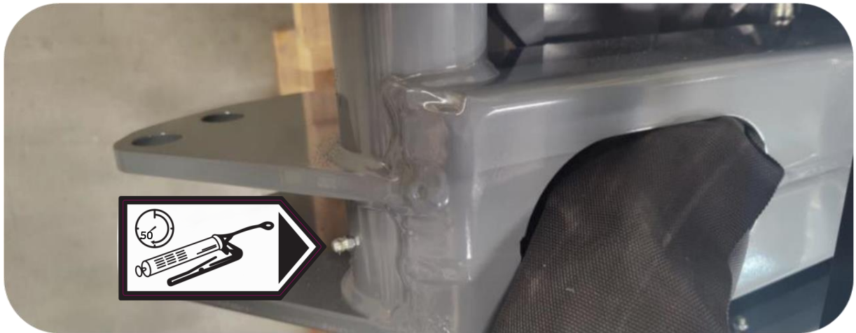
Location of the grease nipple at the inner side of the PUMA 3303 Multi Carrier swing arm
