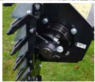
HD PLANETARY GEARBOX WITH CAST IRON ENGINE
