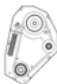
AUTOMATIC BELTS TENSIONER The automatic tensioning system as well as allowing constant power transmission reduces belts wear
