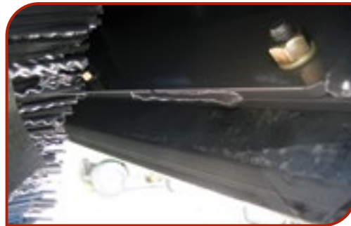
Additional steel reinforcement/welds between bolts and cutting edge and side plates
