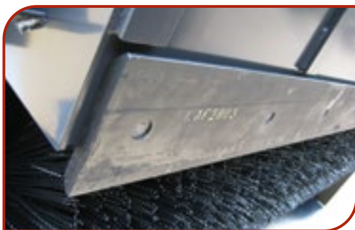
Reversible, heavy duty cutting edge
