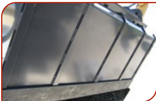
5 wear plates on underside of hopper bin
