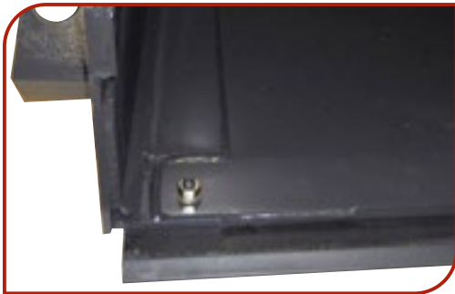
Additional steel reinforcement/welds between bolts and cutting edge and side plates
