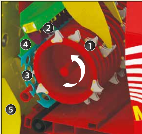
'Dual Chop' mechanism in short chop position
