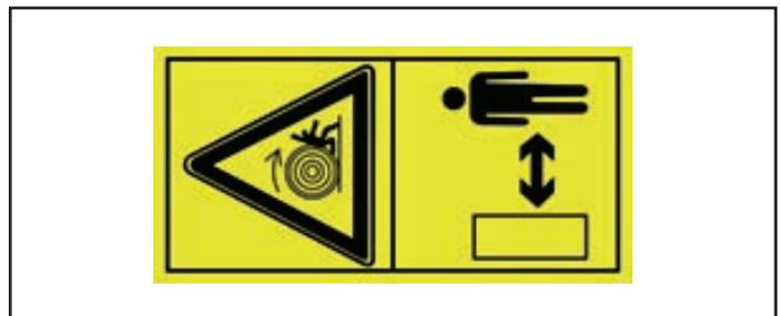
Loading Arm Hazard (Item 7) - Keep a safe distance from the machine during operation.
