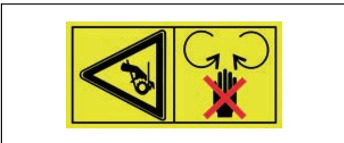
Rotation Hazard (Item 5) - Keep a safe distance from the machine during operation.
