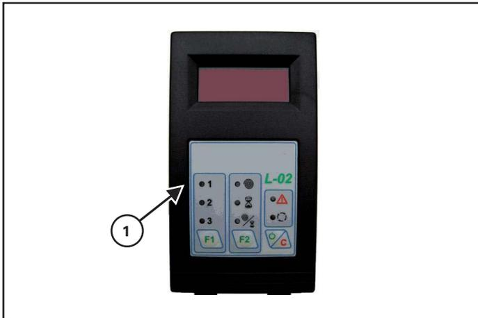
The wrap counter (Item 1) is an electronic device used for counting the wraps on a bale and may be used on all types of wrapping machines. The wrap counter should be installed in the tractor cabin in a place where it is visible and accessible to the operator [Figure 12].
