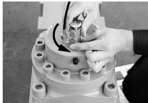
11. Disconnect the charging the adapter
