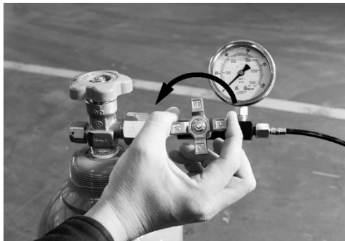
8. Open the 3-way valve slowly and charge the gas (65 kg/cm 2 ). After that, close the valve.
