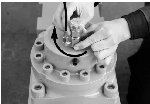
4. Connect the adapter to the inlet of the accumulator.
