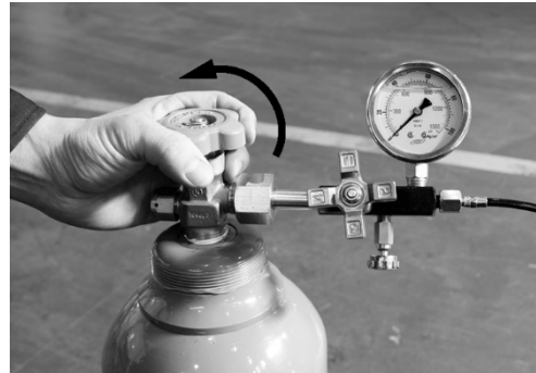
7. Open the valve slowly. Beware of gauge damage if opening quickly.
