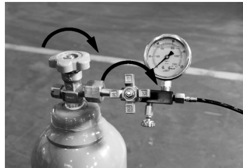
5. Make sure the gas bottle valve and 3-way valve are closed.
