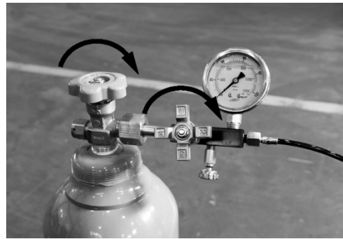
5. Check the gas bottle valve and 3-way which were closed.
