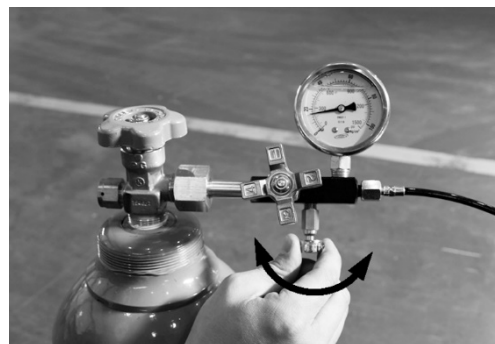
9. Control the proper pressure (55~60 kg/cm 2 ) by opening the drain valve as photo indicates. *Charge the gas considering the temperature in the area.
