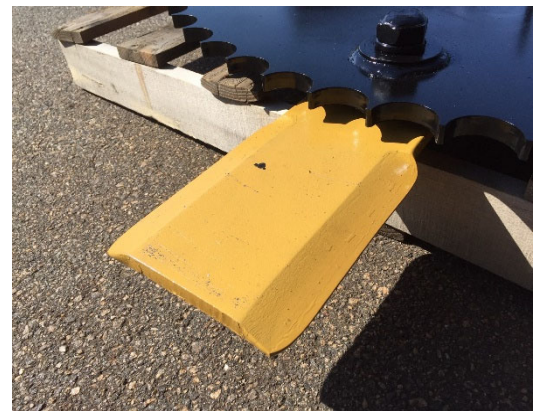
BLADE SHOWN BOLTED TO CARRIER IN CORRECT ORIENTATION WITH TAPERED SIDE OF BLADE FACING UP AND WIDER SIDE OF BLADE FACING DOWN
