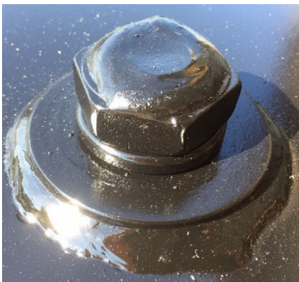
BLADE BOLT SHOWN WITH CONTINUOUS WELD AROUND TOP OF NUT AND BOLT SHANK TO ENSURE THAT NUT STAYS ATTACHED FOR THE LIFE OF THE BLADE
