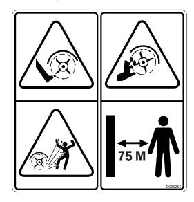
F. D005129 WARNING - Rotating parts hazard. Do not reach into machine. Keep away from machine.
