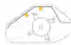
DOUBLE ROWS OF COUNTER KNIVES Increased rows of counter knives hold the material in for more complete shredding
