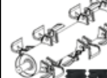
ROTOR "VENTILATOR" electronically balanced. Forest type tool holders moulded in boron steel
