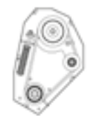
DOUBLE AUTOMATIC BELTS TENSIONER
