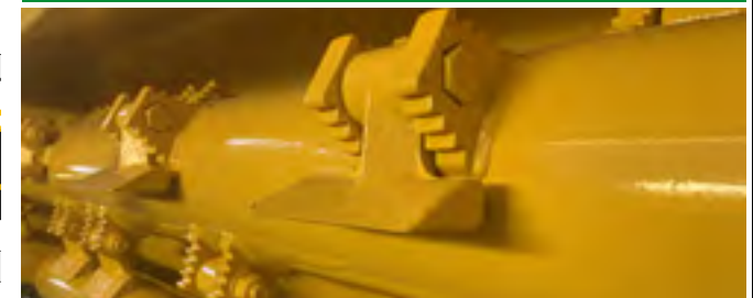
Self-cleaning roller position unloading of mulched product behind the roller for faster working speed
