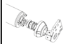
PROFESSIONAL REAR ROLLER Ø 194 mm with 4 taper roller bearings, mud scraper and central body interchangeable with 2 positions: 1) self-cleaning 2) rear (optional)
