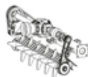
AUTOMATIC TORQUE LIMITER + MECHANICAL CHAIN TRANSMISSION
