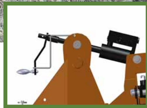
The 4100 was designed to make maintenance easy – with the hydraulic manifold mounted on top of the front tilt cylinder, it makes it simple to check or tighten hoses.
