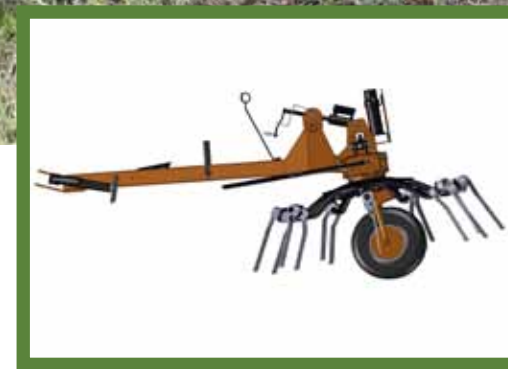
The tongue connects directly to the main tunnel in rear – allowing for smooth and stable tedding.
