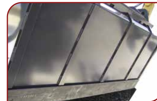
5 wear plates on underside of hopper bin
