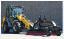
Hydraulic grader attachable to mini-loaders or skid steer loaders. Ideal for spreading material for jobsite ground leveling and preparation.
