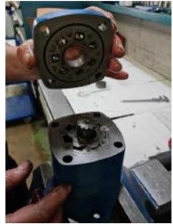
6.- Remove manifold and manifold seals.
