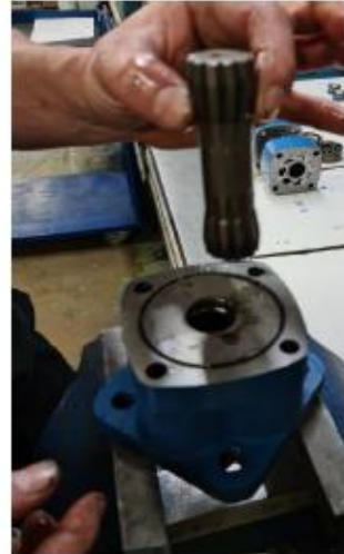
9.- Remove the drive link and it seal.
