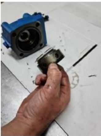
4.- Remove commutator assembly.
