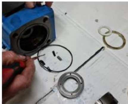
5.- Remove Piston seals and springs.
