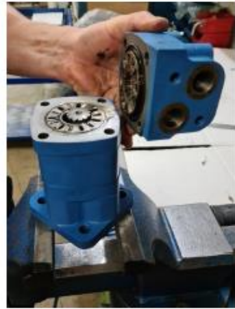
3.- Remove the cover housing and seals.
