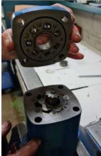
8.- Remove the gerotor and its seal.
