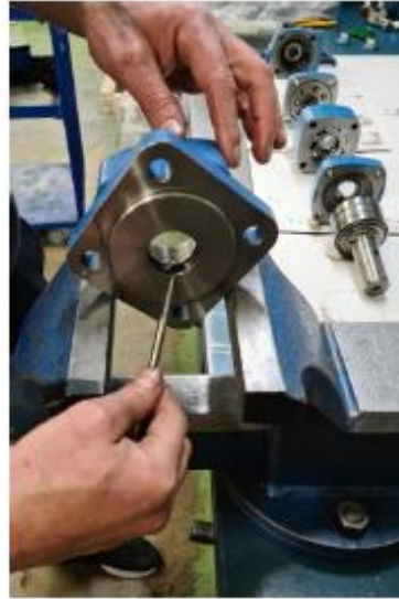
10.- Insert housing and tap out the coupling shaft. 11.- Remove the shaft seal.
