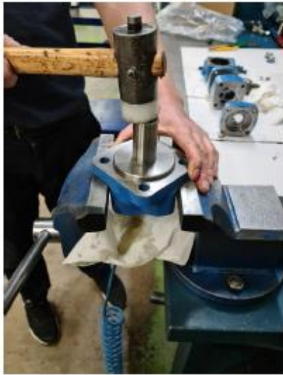
10.- Insert housing and tap out the coupling shaft. 11.- Remove the shaft seal.
