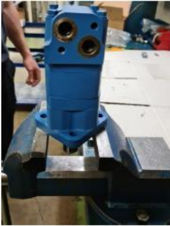
1.- Block the motor with a bracket.
