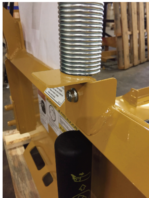
Hose mount assembly, bottom attachment point
