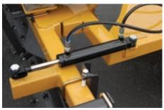
Angling capability powered by the tractor hydraulics
