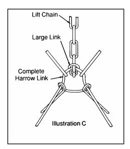
Attach the Lift Chain to the rear bar using 3/8" x 2 ½" carriage bolts, lockwashers and hex nuts. Use the two 3/8" x 1 ½" carriage bolts on the outside holes. Put the bolt through the chain link so that the Harrow lifts completely off the ground when the Lift is raised.
