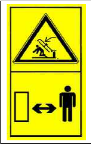
6. Indicates danger caused by accidental fall of suspended arms. Keep safe distance
