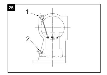
caps 1 (filling and level) and pour in the amount shown or the amount needed to top up the level through the hole in cap 1 (tilt the bar slightly if necessary so it is easier to pour in the oil) until the level of cap 1 is reached.
