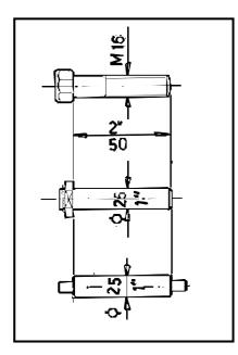
Example: a pin with a 25 mm (1") diameter and a screw with an M 16 (5/8") diameter, both 50 mm (2") long, will be listed as:
