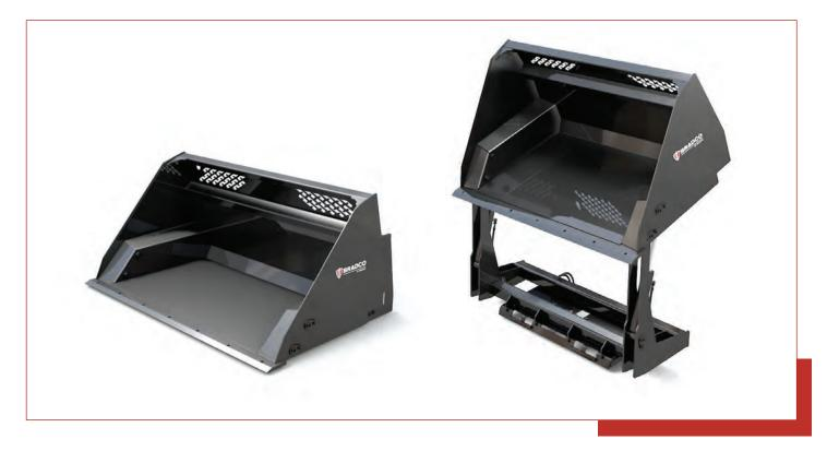
The **Bradco High-Dump** line of buckets allow users to increase the dumping height of their machine by 74 inches and load material into trucks, feed bins and reach other landing heights previously not obtainable with a standard bucket. This light material high-dump bucket exceeds all competitive units by offering increased capacities, cushioned hydraulics, 114° of roll out and the most robust design in the industry. These features translate to higher productivity and faster cycle times.
