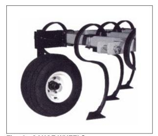
Fig. 8 GAUGE WHEELS (TYPICAL MOUNTING POSITION)
