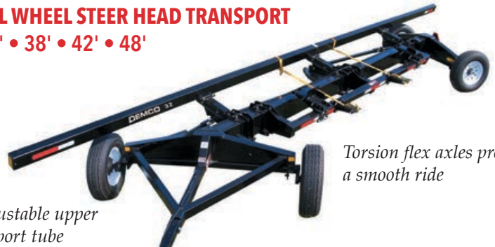
Standard telescoping tongue and EZ Latch 2 5/16" ball coupler and safety chains
