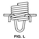
5. To replace the springs, it is necessary to remove the top spring anchor (#814408) and to remove the two lower bolts that hold the lower end of the main hydraulic cylinder. Removing these bolts will allow the removal of the lower spring bracket (#814430 on HPD-16).
