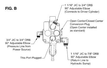
Connect the <sup>3</sup>/<sub>4</sub>" I.D. x 24" long hose from the control valve work port to the Post Driver hydraulic cylinder port.
