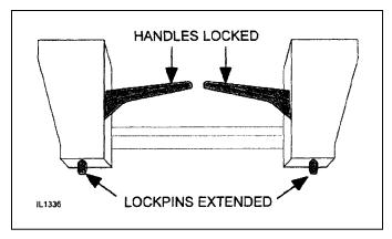
Figure 3. Attachment Coupler Handles - Locked
