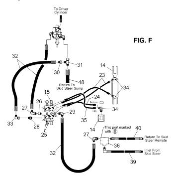
**MOUNT ASSEMBLY:** Connect a 3/8" I.D. x 36" long hose from the inlet side of the ram control valve to the 90° elbow (#27) in the 2 spool valve.
