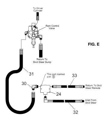
**NOTE:** Hose (#31) and elbow fitting (#30) need to connect to the port of the flow divider valve (#24) marked with a number 8.
