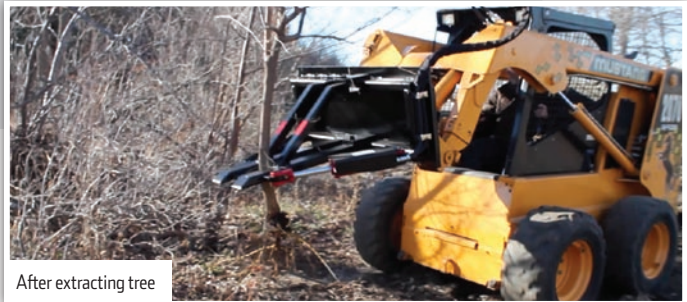
Extractor closing on tree
